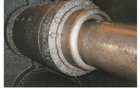
Spindle special seal for harsh environments.
