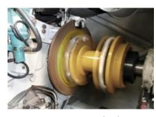
Torque monitoring on wind turbines.
