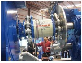
Ixilflex® with JGFS composite spacer.
