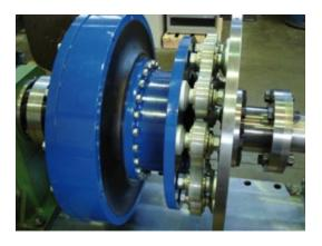
$\label{limits} \textbf{Ixilflex} \textbf{@ combined with a highly elastic coupling.}$
