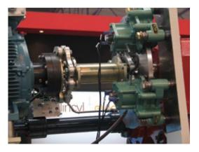
Ixilflex® with torque limiter.
