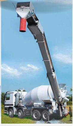
This transport concrete mixer is fitted with a 16.5 m conveyor belt, swivelmounted in two levels, each having a WD-LC 0419 slew drive
