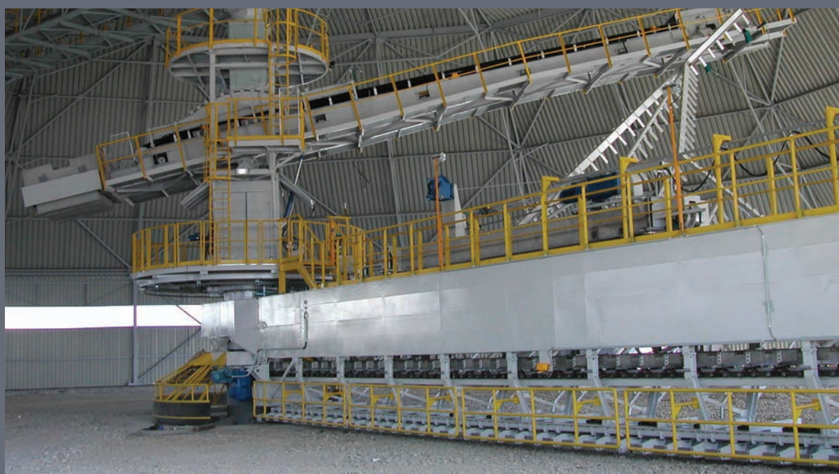
Circular bridge type scraper reclaimer in a limestone storage hall
