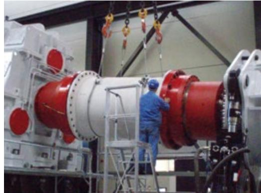
Jaure MTGX-HD-TI-1000/JHC-700 on wind test bench
