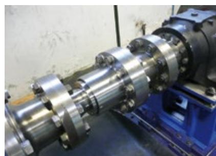
In house fatigue testing JHC-HF-F-100
