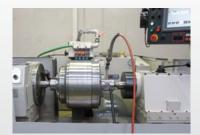
Mounting the regrinding jig and bearing assembly to the cylindrical grinder
