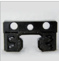
End seal in good condition
