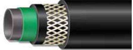
Low-permeation, premium hose for use on carbureted engines, PCV and EEC systems, and for fuel return hose on fuel injection systems. Not for use on the pressure-side of fuel injection systems. Approved for use with leaded and unleaded gasoline, diesel, bio-diesel, E-85, methanol, ethanol, and gasohol fuels. A patented five-layer Greenshield® barrier technology keeps fuel out of the environment while delivering peak fuel efficiency.
