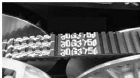
*Although G-Force® belts are not directionally biased, it is recommended to install them with the label lettering facing toward the user to keep belt reinstallation consistent*
