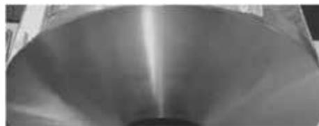
*Dirty sheaves should be cleaned with a mild abrasive to remove rubber and other wear contaminates, as shown above by Dirty Sheave Plates. Dark wear patterns must be removed from the surface then cleaned off with an alcohol or brake cleaner to remove fine particulates.*
