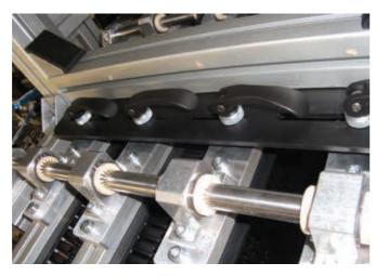
The production line should be adjusted without setup time being required. drylin® linear guides, which enable precise and fast adjustment, were used for this.
