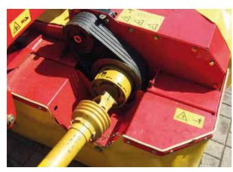
The conventional roller ball bearings were replaced by iglidur® plain bearings. The plastic bearings are corrosion and dirt resistant.
