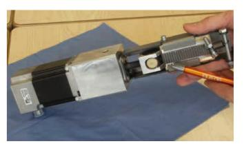
Anti-backlash lead screw nuts in a glue application system of a seam gluing machine (wood industry). These ensure the utmost precision for this clearance-free adjustment drive.
