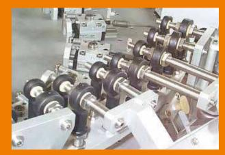
igubal® rod end bearings made from plastic display their strength in the demanding environment.
