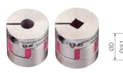
The coupling connects the drive shaft of the axis to the motor. An elastic polymer insert in the centre of the coupling transfers the motor torque. This damping element compensates for radial and axial clearance.
