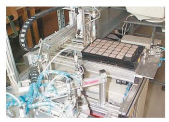
The removal unit is moved along the X-Y axis using the space-saving and cost-saving drylin® N lowprofile guide. The rugged drylin® T guide system undertakes the vertical guidance.
