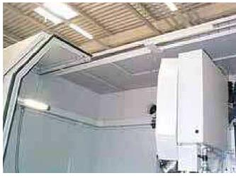
The smooth, low noise operation and the enormous cost advantages are obtained by the use of the drylin® linear bearings on the hard-anodised guide shaft to guide the doors of machine tools.
