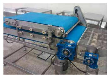
Corrosion resistant iglidur® bearings in use in a meat roller - also resistant to aggressive detergents.
