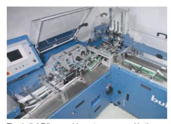
The drylin® T linear guide systems are used in these enveloping machines to guide an envelope suction opener that is mounted on one side.
