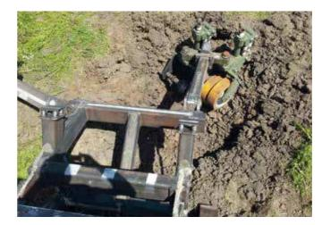
iglidur® plain bearings were used for mounting the wheels and the join arm of the wheel set, unlike metal bearings, they are resistant to dirt and humidity.
