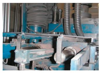
By changing over to the drylin® R linear bearing, the maintenance rate of this compaction unit could be extended by 2 years, despite high stressing from powder particles and abrasive agents.
