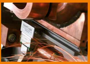
drylin<sup>®</sup> linear guiding system in the EURO-C welding tongue for the automotive industry.
