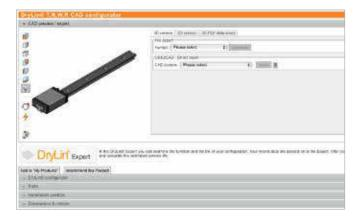
For nearly all igus® products, CAD data are available for downloading free of charge. Simply choose a product group, call up a CAD model, select 2D or 3D output, and generate. You can download all generated CAD files via the download centre or transfer them directly to your CAD system by clicking on "Click2CAD".
