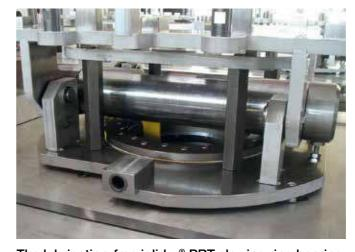
The lubrication-free iglidur® PRT slewing ring bearing masters this job brilliantly, is lighter and in terms of purchasing is more affordable than a comparable metal rotary connector.
