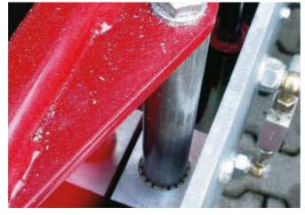
Saw mill: linear guide with iglidur® J plastic liner for the angle stops. The iglidur® J is best suited for most linear applications due to its low wear and low friction properties.
