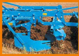
No lubrication necessary in the overload element of carat 9 (intensive grubber).
