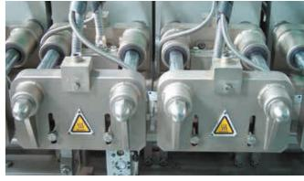
FORMING, FILLING AND SEALING MACHINE Lubrication-free drylin® high temperature bearings (up to +120 °C) are used in the tool guide system of this forming, filling and sealing machine. (Unifill SpA, Italy)
