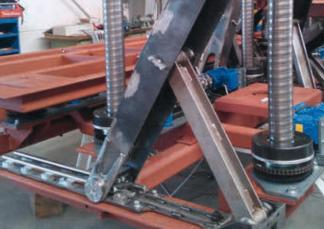
Quiet, low vibration adjustments in the stage technology field are enabled through the use of drylin® W linear guide systems based on steel shafts in combination with stainless steel housing bearings.
