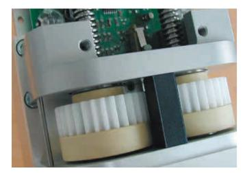
This mixing station uses two drylin® trapezoidal lead screw nuts made from iglidur® high performance polymer for the optimal mixing ratio of a two component silicone mass.
