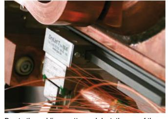
Due to the welding spatter and dust, the use of the extremely dirt-repellant drylin® T linear guide system finds the balance between high service life and low costs.
