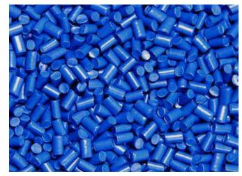
Picture 04: Polymer granulate; basis compound of the lubrication-free and predictable iglidur® bearings
