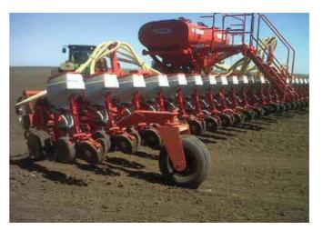
Dust and humidity mean a high degree of wear in the contact zone of the swivelling wheels of this planting machine. iglidur® Z thrust washers resolve the problems.
