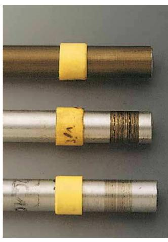
Picture 9: Wear experiments with aluminium shafts
