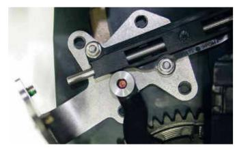
By using wear-resistant iglidur® clip bearings, the lowering mechanism for radiator mascots on luxury cars could be improved.
