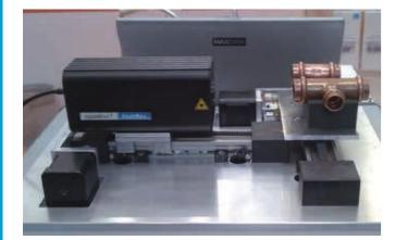
ADJUSTMENT OF INSPECTION EQUIPMENT drylin® ZLW toothed belt axis in the inspection camera adjustment for the position inspection of sealing rings. (OLPE Jena GmbH)
