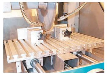
drylin® R linear bearings on supported aluminium shafts are used in this grinder to guide the cutting
