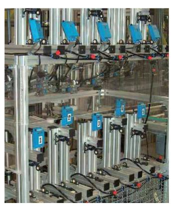
Picture 12: Oscillating wear test rig for testing the wear in oscillating movements at medium loads
