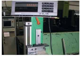
Major time savings: the measurement system makes tool changes far quicker. The gauge runs on a drylin® T rail. This solution also works seamlessly in dusty environments.
