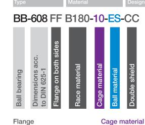
F: Flange on one side FF: Flange on both sides Race material **F180:** xirodur® F180 **B180:** xirodur® B180
