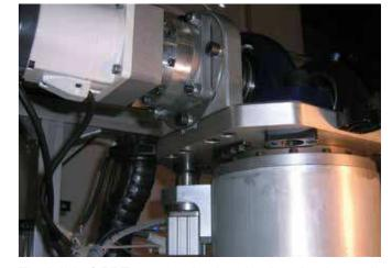
The iglidur® PRT-01-100 slewing ring bearing is used in an automatic welding plant in this application. It enables pivoting in the horizontal plane of the clamping device.
