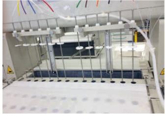
The sampling device uses drylin® linear bearings to remove the products precisely and smoothly.
