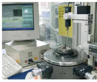
Picture 13: Measurement of the inner diameter of a press-fit plain bearings
