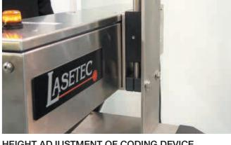
HEIGHT ADJUSTMENT OF CODING DEVICE
