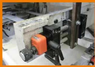
Lead screw unit with accessories ensures speedy, precisely repeatable format adjustments.
