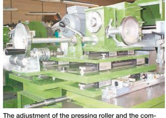
The adjustment of the pressing roller and the compensation of the imbalance of the grinding tools are implemented here with drylin® T in place of recirculating ball-bearing guides.
