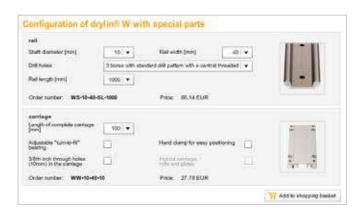
Assemble double rail and carriage to your requirements. You receive the systems without mounting holes or already machined. drylin® W profile rails with standard holes or without holes can be delivered in one piece up to 4,000 mm long – Your required length is cut to size. drylin® W profiles with 3/8" threaded holes are available, also available in fixed lengths of 1,000/1,500 mm.
