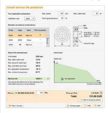
The xiros® service life predictor calculates quickly and easily the expected service life of the xiros® plastic ball bearings specifically designed for your application. This xiros® service life calculator is continually being supplemented with new values and xirodur® materials.
