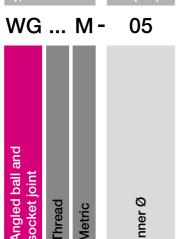
Thread L = left-hand thread R = right-hand thread Ball stud Blank = plastic stud MS = ball studs made from galvanised steel19) ES = ball stud made from Stainless steel<sup>28)</sup>
