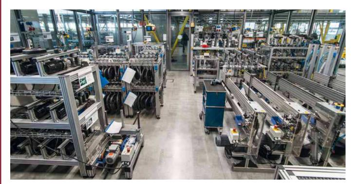
igus® lab: 15,000 tribological tests (friction and wear) in 300 test set-ups in the industry's largest laboratory (2,750m²). View inside bearing laboratory in Cologne.
