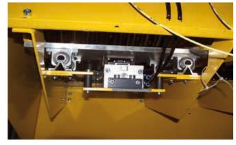
Cost-effective guide for work piece carriage in a machine tool through supported aluminium shaft.
