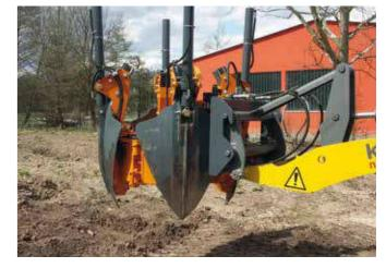
The spades are pushed slowly into the soil. The polymer plain bearings are able to deal with dirt, moisture, etc.
