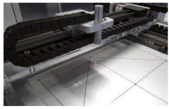
SENSOR ADJUSTMENT/MEASURING SYSTEMS drylin® ZLW-0630 toothed belt axes as a two-dimensional linear robot (X,Y axis) to adjust a laser measuring head. Compact, lightweight and maintenance-free due to polymer plain bearings.
