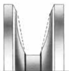
Worn Groove Sidewalls
