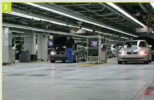
Illustration 3: Slat conveyor in the finishing area and fluid filling, with staff stand- ing on the conveyor
