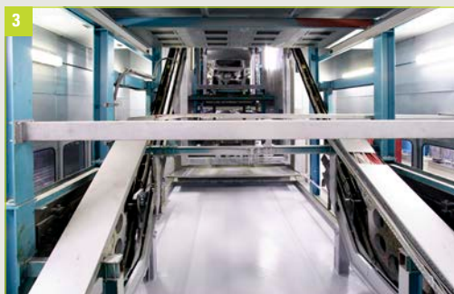
Illustration 3: Pendulum conveyor chain in the Cataphoretic Painting dip tank
