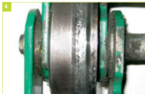
Illustration 5: Lube-free double- strand chain with inside mounted rollers
