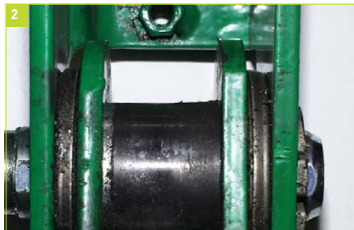
Illustration 3: Lube-free double-strand chain with outside mounted rollers
