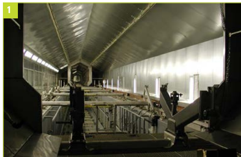
Illustration 1: Rotation tunnel with rotary axles and RoDip chains at each end
