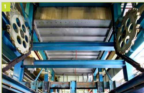
Illustration 2: Sprocket with exchangeable tooth gaps
