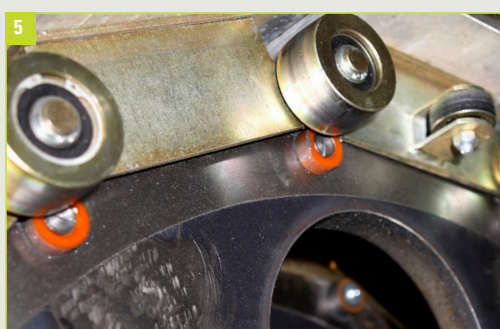
Illustration 5: This slat conveyor chain in the Conservation area is operated in intervals with a speed of up to 40m/min. The sprockets are equipped with the patented KettenWulf noise dampening system.
