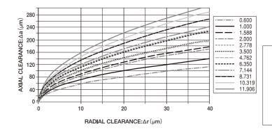
$\Delta a = 2\sqrt{\Delta r(r_0 + r_i - Da)}$  (mm)
