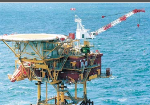
Offshore lattice boom crane
