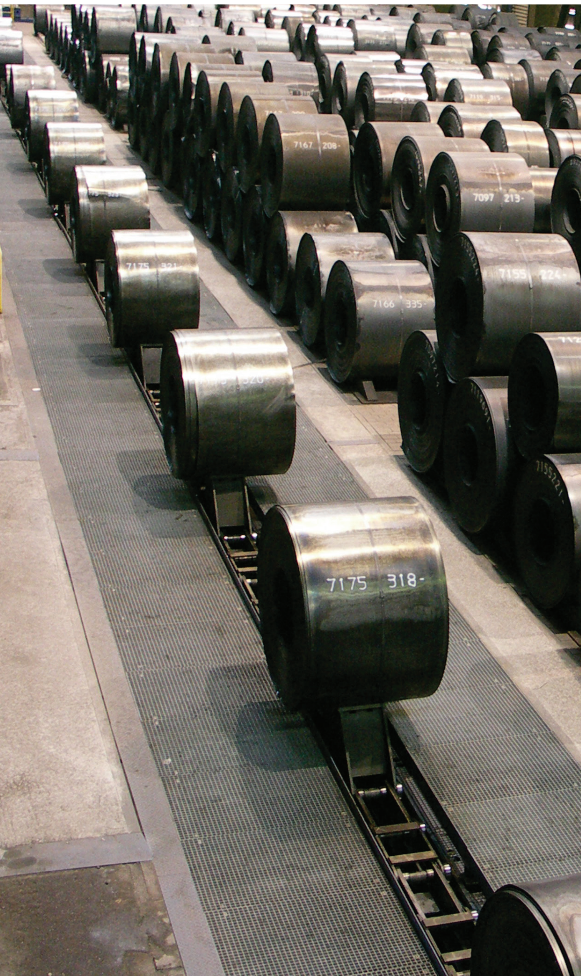
KettenWulf chain technology for coil conveyors with center distances of more than 100 meters and total loads of more than 700 metric tons.
