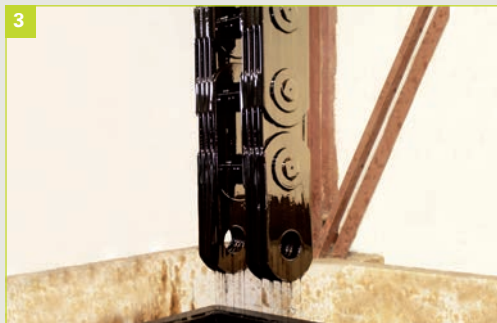
Illustration 3: Lubrication by submerging in a special oil bath
