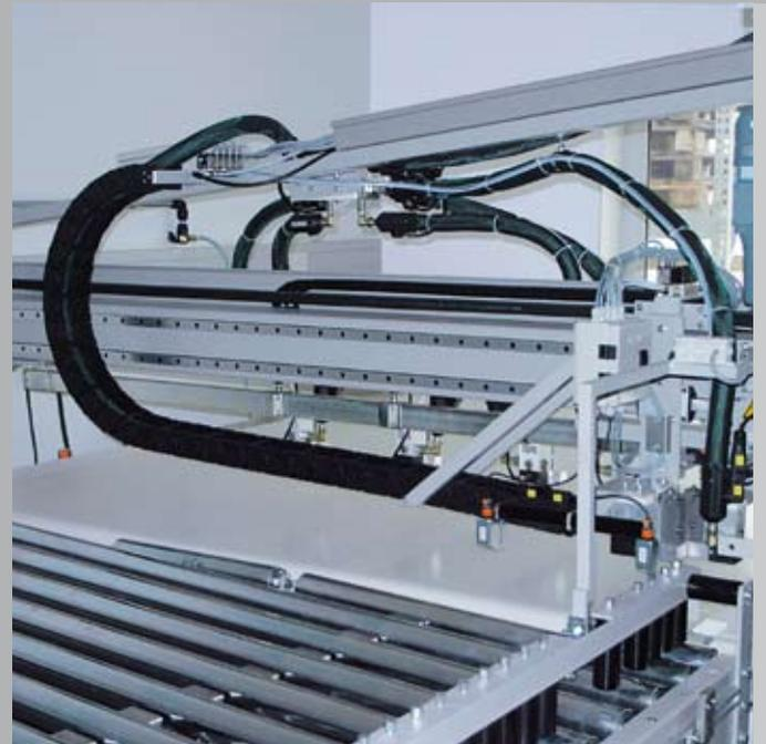
The Franke Dynamic Aluminium Roller Guide is also used on packaging machinery for mattresses. In addition to cleanliness, the mobile function of the guide unit must be ensured, to avoid soiling the mattresses.
