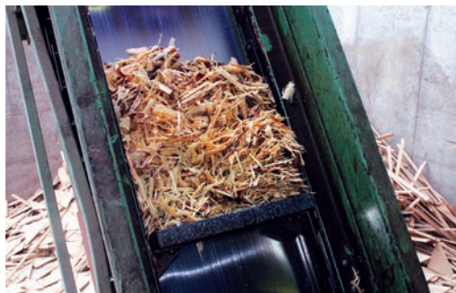
Wood chips conveyor at root reducer and trimming station
