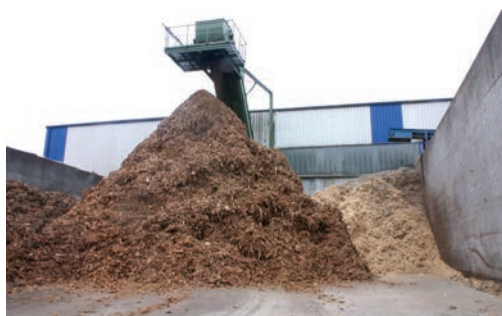
Wood chips conveyor at debarking station
