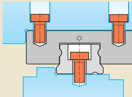
The illustration opposite shows the ideal mounting arrangement for miniature profile rail guides. Carriage and rail can be mounted at both sides, but their datum planes should be on the same side of the system. To ensure a neat abutment to the adjacent edges, these should feature a relief fillet.
