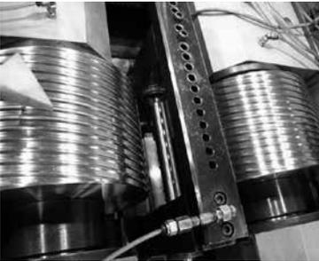
We employ the most advanced digital electric screw thread rolling machine. During the manufacturing process, the oil cylinders on the two axes of the thread rolling dies employ a servo hydraulic system for the correction of oil pressure and positioning precision.
