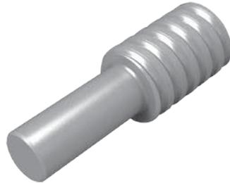
Fig. 3.6.2 Through end thread
