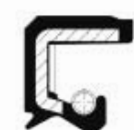
AS - PX Reinforced sealing lip and special metal insert for overpressure, with additional dust lip
