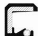
A - FL Different spring groove for a better spring retention
