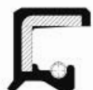
AS - P Reinforced sealing lip for overpressure, with additional dust lip
