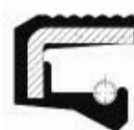
A - X7 Wavy rubber covered O.D., metal insert, sealing lip with garter spring
