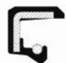
A - P Reinforced sealing lip for overpressure
