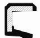
A - O Sealing lip without spring
