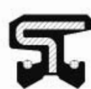
A - DUO Twin sealing lip with two garter springs
