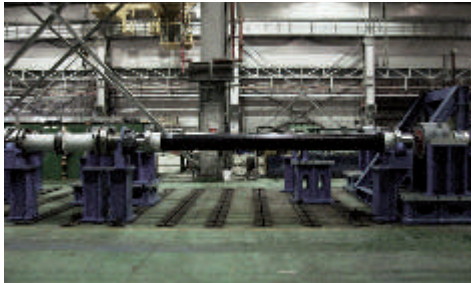
Carbon Fibre Shaft combined with LAMIDISC® coupling
