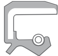
Double lip with spring Dos labios, con resorte
