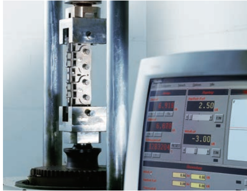
Figure 1: The high-frequency pulsometer determines the fatigue strength
