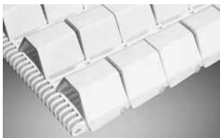
SERIES 600 • Center-driven • Closed hinge • 2.00 in. (50.8 mm) pitch • Non flush edge
