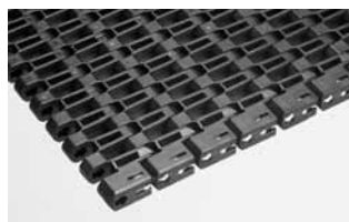
SERIES 1700 • Center/Hinge-driven • Closed hinge • 1.50 in. (38.1 mm) pitch
