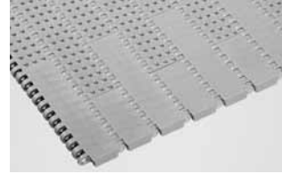
SERIES 900 NUB TOP • Center-driven • Open hinge • 1.07 in. (27.2 mm) pitch
