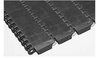
SERIES 900 • Center-driven • Closed hinge • 1.07 in. (27.2 mm) pitch
