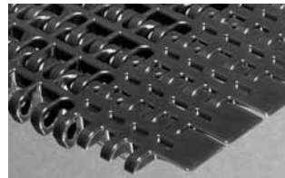
SERIES 1100 Flush Grid • Hinge driven • Open hinge • 0.60 in. (15.2 mm) pitch • Available width: 4 in. (76 mm) and up in 1.00 in. (25.4 mm) increments and 6.0 in. (152 mm) MTW
