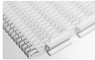
SERIES 2000 • Center-driven • Open hinge • Sideflexing • 1.25 in. (31.8 mm) pitch
