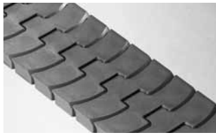
SERIES 4014 Flat Top • Hinge driven • Closed hinge • Sideflexing • 1.00 in. (25.4 mm) pitch • Available width: 83.8 mm (for parallel running at 85 mm)
