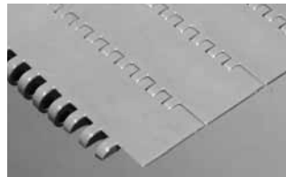
SERIES 900 Flat Top • Center-driven • Closed hinge • 1.07 in. (27.2 mm) pitch • Available widths: 4.7 in. (119 mm) and 6.0 in. (152 mm)
