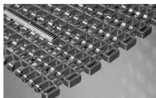
SERIES 2600 RFT • Hinge-driven • Open hinge • Sideflexing • 2.00 in. (50.8 mm) pitch
