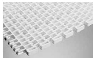
SERIES 2600 (3.2) • Hinge-driven • Open hinge • Sideflexing • 2.00 in. (50.8 mm) pitch
