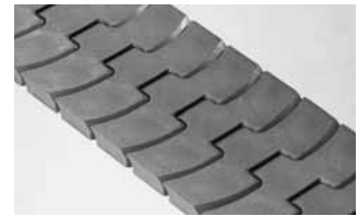
SERIES 4009 Flat Top • Hinge driven • Closed hinge • Sideflexing • 1.00 in. (25.4 mm) pitch • Available width: 83.8 mm (for parallel running at 85 mm)
