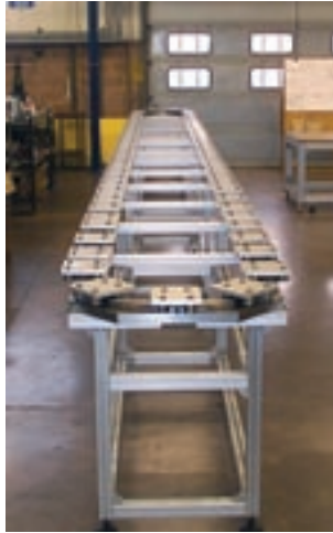
The stainless steel HepcoMotion PRT provides smooth motion and high stopping accuracy and reliability for this continuously indexing automated filling line. The PRT operates 24 hours per day and runs completely dry to avoid contamination.
