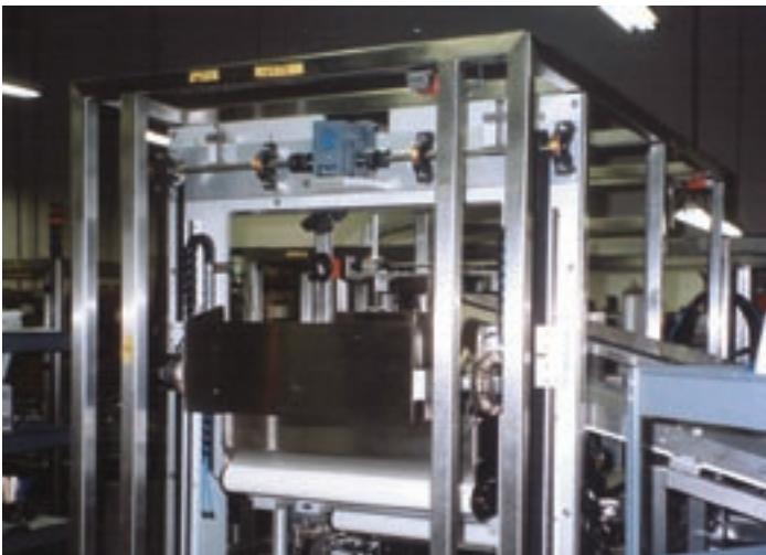
DualVee wheels and pre-mounted track plates provide an effective and compact method to raise, lower and guide a bucket full of products from one conveyor line to another for this pharmaceutical, cosmetic and personal care packaging machinery.
