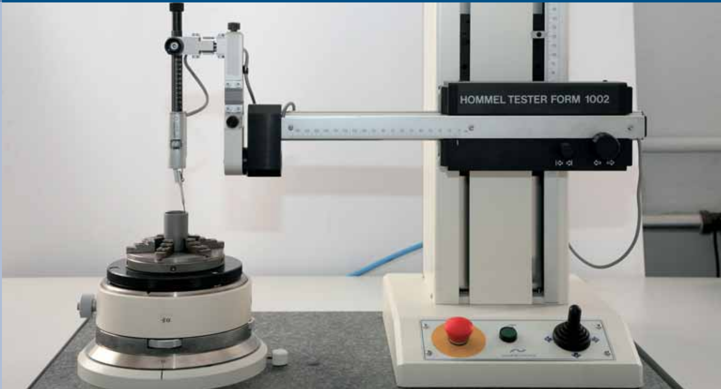
Shape measurement of chain components
