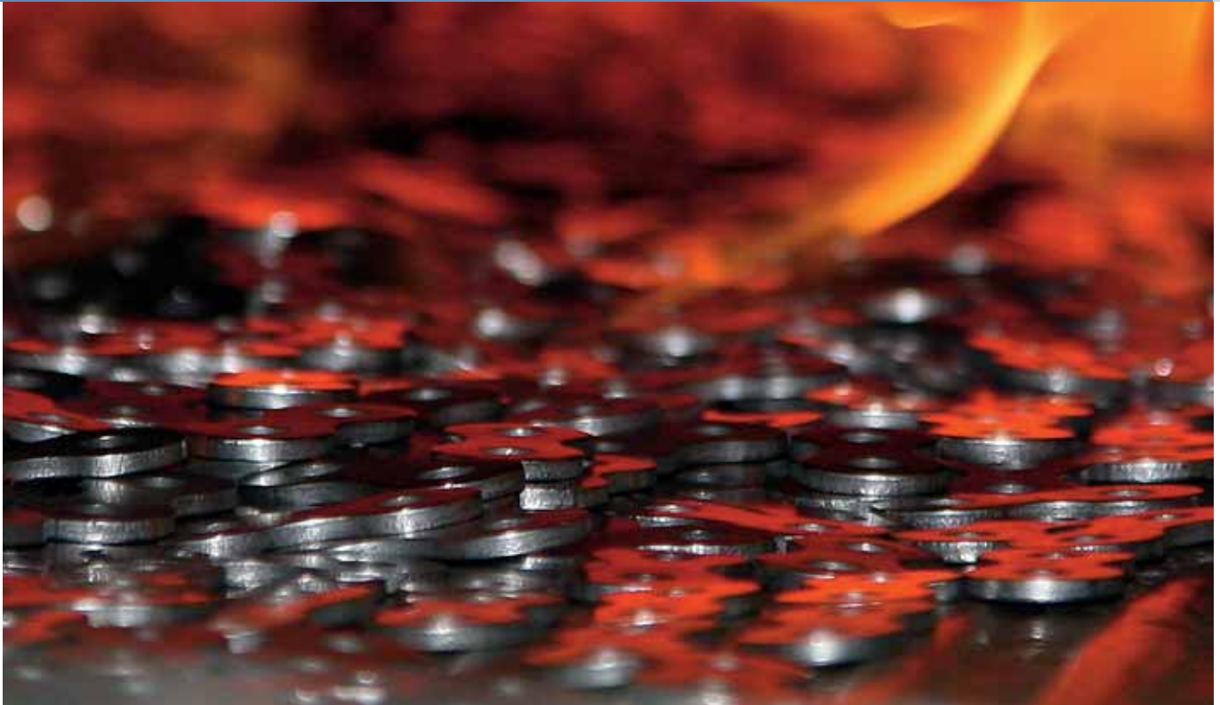
Chain plates in the continuous annealing furnace
