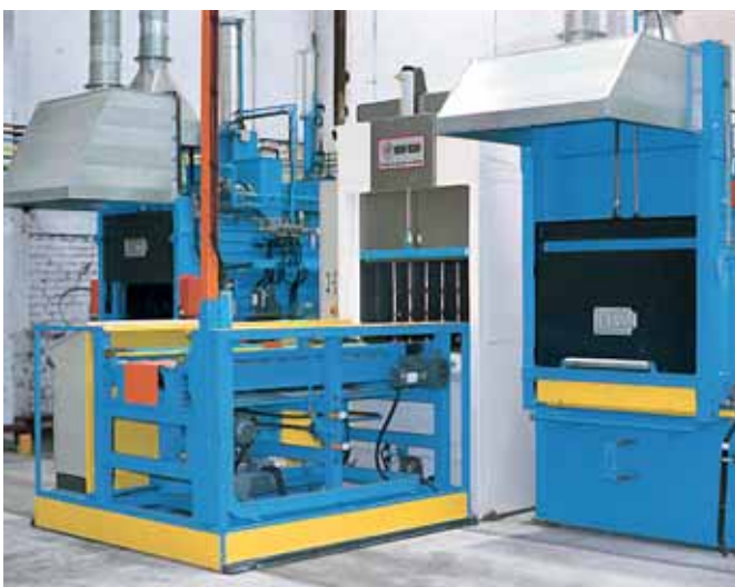
Sophisticated equipment for heat treatment: chamber kiln
