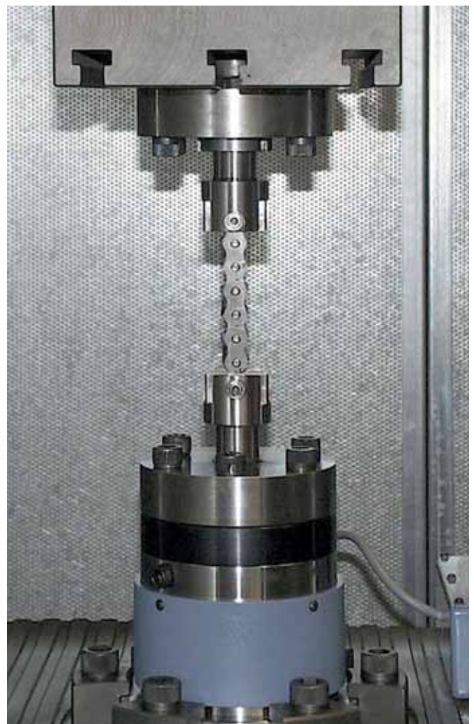
Quality checks with state-of-the-art test stands: fatigue resistance test
