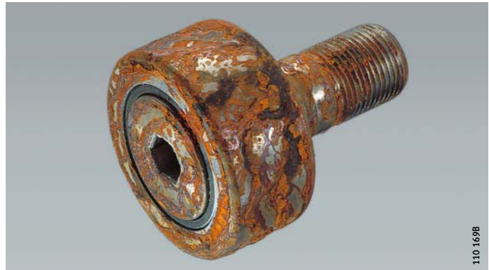
Figure 1 NUKR52 without coating after salt spray test
