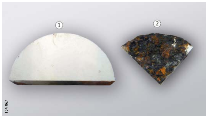
Figure 2 Corrosion resistance, comparison after 500 h in salt spray test
