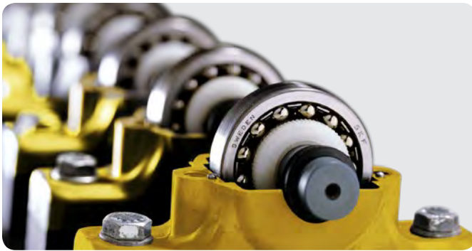
Emcor grease test rig
