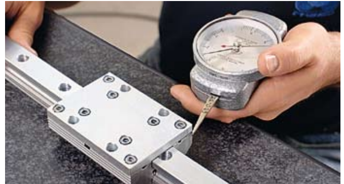
Illustration 2: Measuring Slide Resistance
