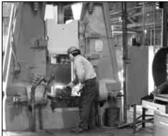
One of the many hammers capable of producing forgings up to 50 lbs.
