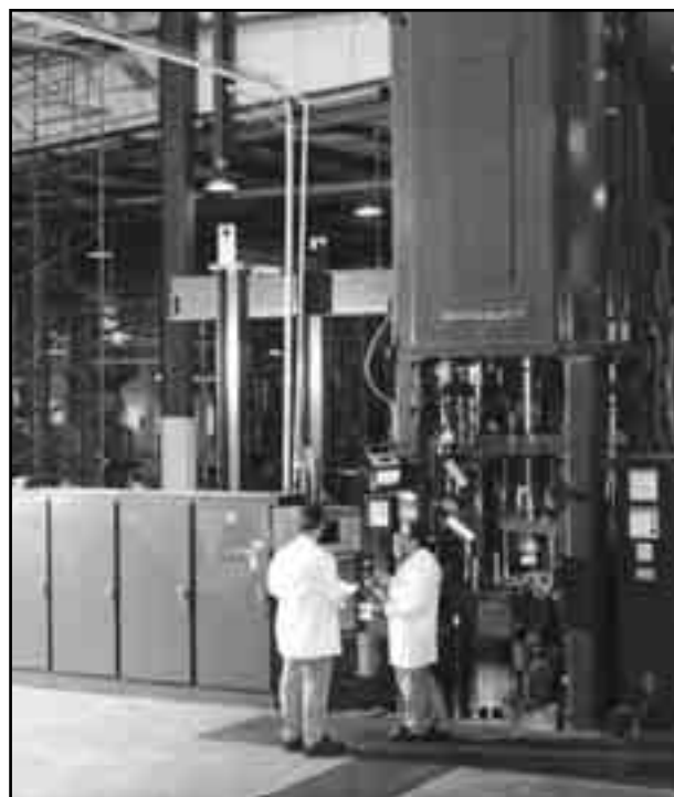
Presses delivering more than 880 tons of pressure form parts from bronze, iron, copper, manganese, etc.
